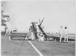
MOVEMENT OF aircraft from the flight deck to the hangar deck, below the flight deck, is done by two elevators at either end of the ship. When up, the platform of the elevator becomes a solid part of the flight deck. The carrier's detection and navigation gear towers above the deck. MOVIMENTO DI avion for di dek di vuelo pa dek di hangar, cual ta haa di e dek di vuelo, ta worde efectua pa medio di dos lift, na cada banda di e Karel Doorman.
